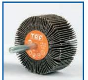
This range of flapwheels are made in aluminium oxide semiflexible cotton cloth (XF backing). They are designed for grinding, deburring and polishing of intricate surfaces, small components, external pipe finishing.
