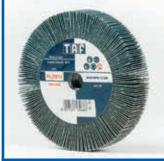
These products are used on portable angle grinders. Suitable for removing welds on irregular surfaces. Ideal for pipes finishing. Recommended for applications on stainless steel. Equipped with M14 threaded bore to be mounted on angle grinders.
