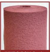
118 is an open structure aluminium oxide non-woven nylon fibre. It is used for light deburring and satinizing of metals with a low stock removal. Water and oil resistant.
