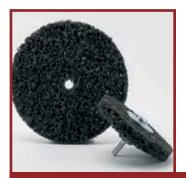
Politaf Dark is a non-woven nylon product impregnated with abrasive mineral. It is mainly used for rust removal, cleaning of worn surfaces, weld seams, moulds, etc. The flexible and elastic structure grants an exceptional cleaning performance without damaging or modifying the original shape of the workpiece. Suitable for stationary machines. Mandrels are required for mounting on portable machines.
